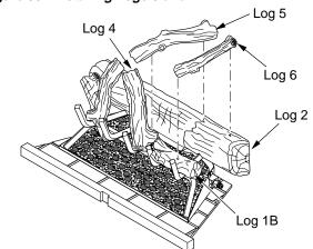
Figure 31 - Installing Logs 5 and 6
